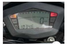
A picture is worth 1000 words-or in this case, 10,000 miles. Check-engine light stayed on after we removed the stock exhaust system with its power valve.
