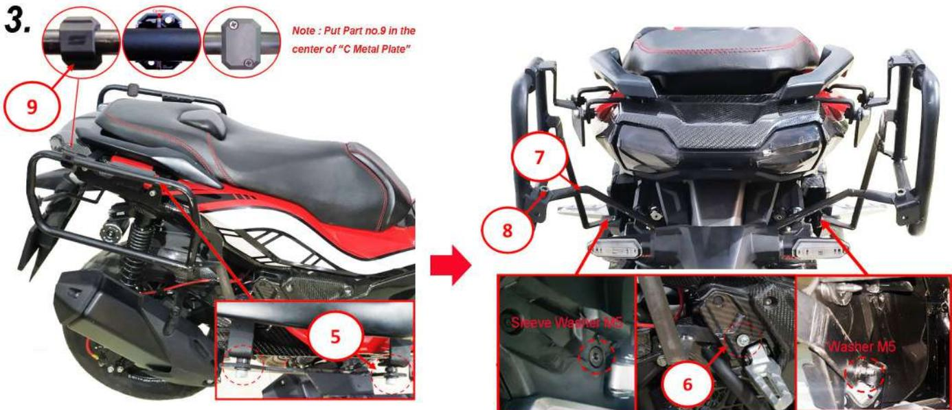
Install the 4P kit in to motorbike ( Ensure left and right bracket position are symmetric ) by using part no.5,6,7 and 8. Install part no. 9 to 4P bracket.
