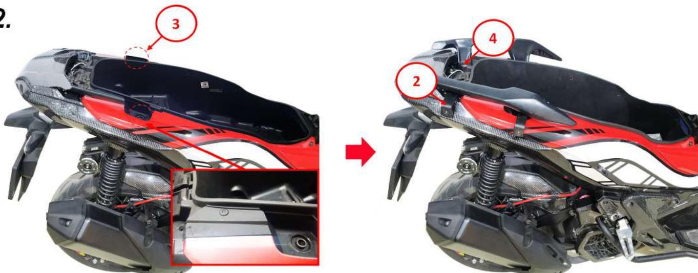
Put part no.3 in to motorbike then Assembly part no.2 ( Short metal part in front and long metal part in rear ) by using part no.4
