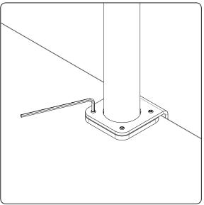
4. Tighten 4x screws - starting with the 2 at rear - with provided hex key clamping the monitor bracket onto your MOVI workstation.
