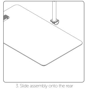
3. Slide assembly onto the rear edge of desk, centering the monitor to your workspace
