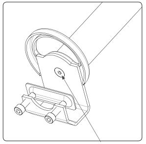
1. Remove post from CME assembly by removing screw in base of post. Keep screw for re-use in step.
