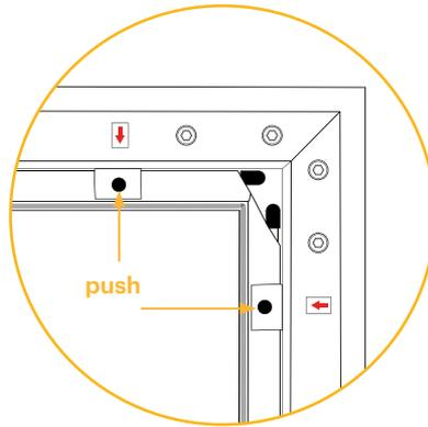
**NOTE:** When pinning the screen fabric to the frame, make sure to pin the four (4) corners of the screen to the frame first so that the screen is properly stretched out and spread along the frame. Then, pin the sides of the screen fabric to the frame.
