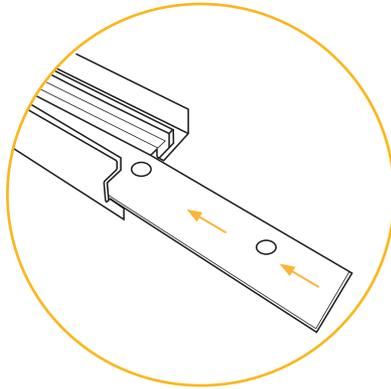
3. Slide the plastic screen pins into the rails on the horizontal and vertical frames. Use the red arrows to place the screen pins in the designated position.
