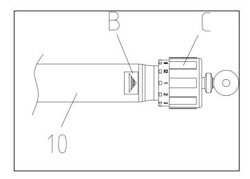
To adjust the tension level, turn the **Adjustment Knob (C)** on the **Hydraulic Cylinder (No.10)** to the desired level. The tension levels range from Level 1 to Level 12, with Level 1 being the lowest resistance. The number pointing to the **Adjustment Knob (C)** by the **Arrow (B)** is the resistance value of the current **Hydraulic Cylinder (No.10)**.
