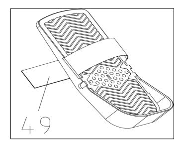
The **Pedal Strap (No.49)** is adjustable and can be personalized to fit the user's foot size.
