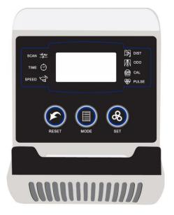
**BATTERY:** The computer uses 2 AAA batteries, which are included. If there is a problem with the display, try changing the batteries first. When changing the batteries, change both of them. Do not mix old and new batteries. Do not mix battery types. Dispose old batteries according to your regional guidelines.
