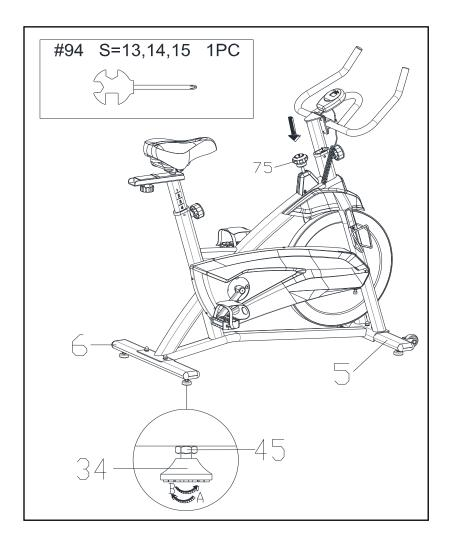
To achieve a smooth and comfortable experience, you must ensure that the bike is stable. During use, if you notice that the bike is unbalanced, you can adjust the **Base Levelers (No.34)** located beneath the **Front & Rear Stabilizers (No.5 & 6)**.
