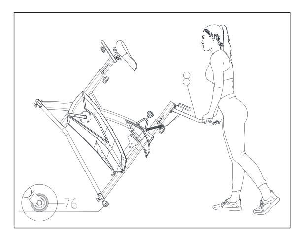
Firmly grasp and hold each side of the **Handlebar (No.8)**. Place one foot on the front base and tilt the bike towards you until the **Transport Wheels (No.76)** on the front base touch the ground. With the **Transport Wheels (No.76)** on the ground, you can transport the bike to the desired location with ease.
