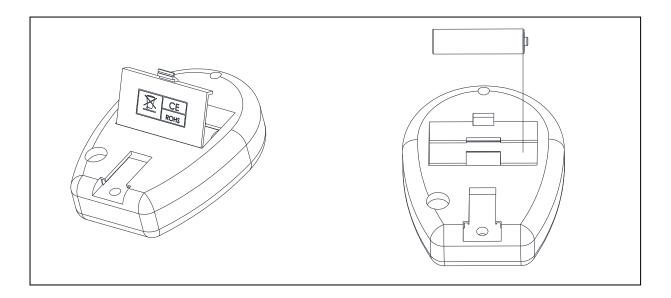
The computer uses 1 AAA battery. If there is a problem with the display, try changing the battery first. The battery is located on the back of the computer.
