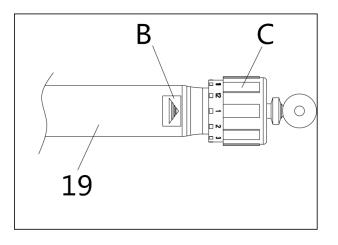
To adjust the tension level, turn the **Adjustment Knob (C)** on the **Hydraulic Cylinder (No. 19)** to the desired level. The tension levels range from Level 1 to Level 12, with Level 1 being the lowest resistance. The number pointing to the **Adjustment Knob (C)** by the **Arrow (B)** is the resistance value of the current **Hydraulic Cylinder (No. 19)**.
