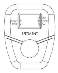
TOTAL CNT (TOTAL): Displays the total number of strokes since battery installed.
