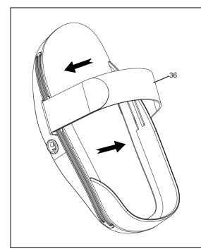
The **Pedal Strap (No.36)** is adjustable and can be personalized to fit the user's foot size.
