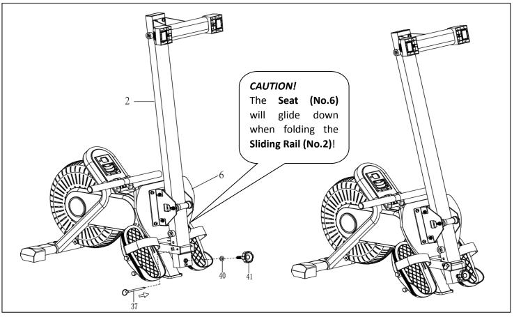
When not in use, you can save space by folding the Sliding Rail (No.2).
