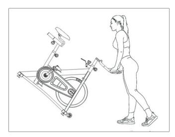
To move the bike, first ensure that the handlebar is properly secured. Then firmly grasp and hold each side of the handlebar, place one foot on the front base and tilt the bike towards you until the transporting wheels on the front base touch the ground. With the wheels on the ground, you can transport the bike to the desired location with ease.
