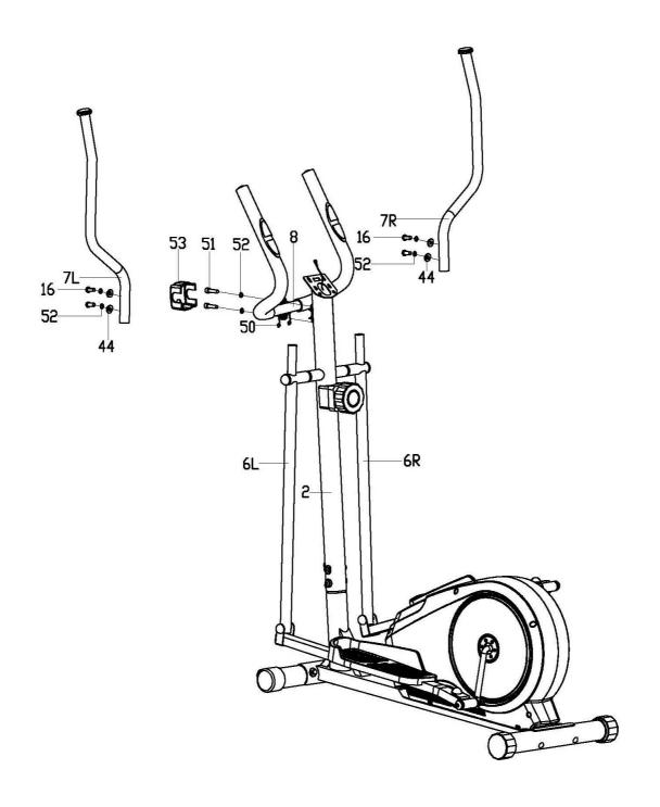
A: Remove Cross Pan Screws (55) from the back of the Computer (9). Connect the Extension Sensor Wire (18) and Pulse Wire (50) with wires of Computer (9) and then fix the Computer (9) to the bracket of Handlebar Post (2) with Cross Pan Screw (55).
