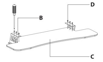
Attach the **Brackets (B)** to the **Keyboard Tray (C)** with **Screws (D)** using a Philips head screwdriver.
