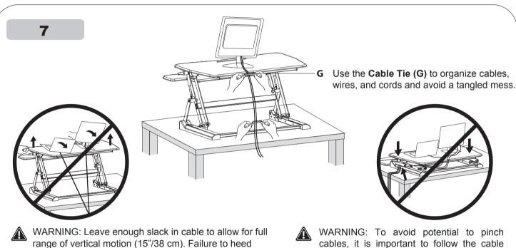
DO NOT place hands on or near support bars. Pinch points are created during lifting and lowering the worksurface. Failure to follow these instructions may result in serious personal injury.
