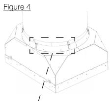
Fasten ductwork to transition using hooks and latches
