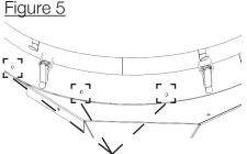
The transition cone can be detached from the backdraft damper by unscrewing the phillips head screws connecting the two.
