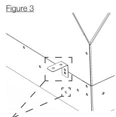
Secure transition to framing using wood screws at the mounting brackets and pilot holes
