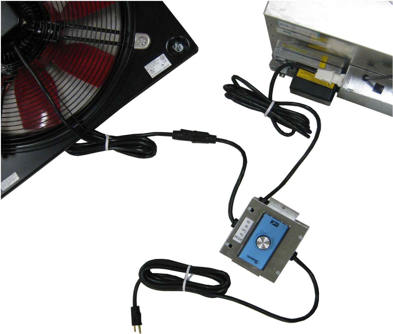
FIGURE 9 – Low Speed controller Installed
