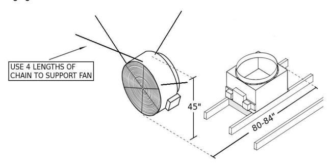
Slide one end of the flexible duct over the damper box collar and fasten with 4 sheet metal screws (see image below).
