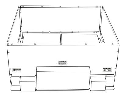
9. Using the provided 2 inch wide foil tape, firmly tape along the bottom seam and all 4 side seams on the interior of the unit. Make sure tape is securely attached and will not interfere with the operation of the damper doors when they open.
