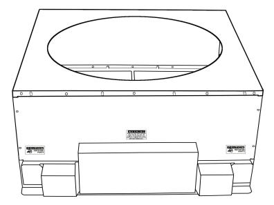
11. Place the damper Collar **E** over the opening on top of the damper and align the screw holes. Attach the collar using the 12 provided collar screws.
