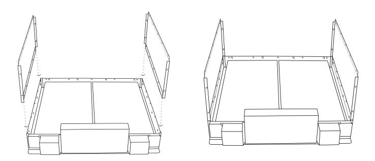
3. Attach the bottom seams of side panels to the base using the provided screws (5 per side). Do not over torque. **NOTE:** We recommended using a manual flat head screwdriver instead of a cordless screwdriver to avoid over-tightening & stripping.
