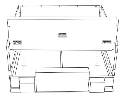
8. Insert 2 plastic rivets along each side seam. Use a hammer to set as before. Remove the electrical box cover and attach the front panel to base using 2 of the provided screws at pre-drilled holes located inside the electrical box.
