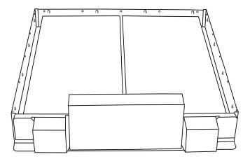
2. Slide both the side panels labeled **A** into the base as shown. Be sure panels slide into the locking tabs on the base. The "A" label must be facing the interior of the damper on both sides.
