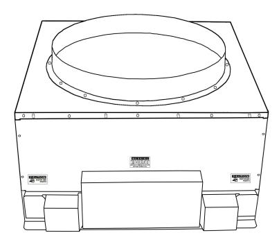
Use the remaining 2 inch foil tape to tape around the outside of the upper seam of the box and around the base of the damper collar.
