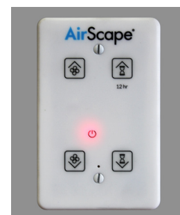
Connect the CAT5 cable. Mount the faceplate to the bracket with the provided white faceplate screws
