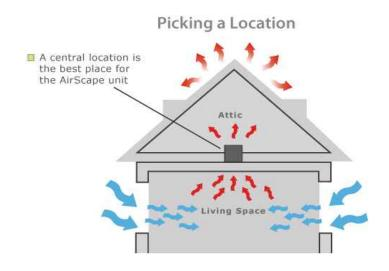
Installing the unit centrally ensures air is replaced evenly throughout your house
