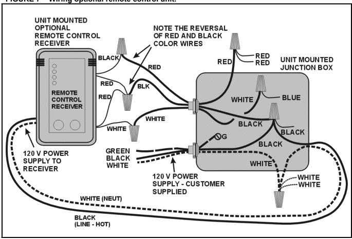
FIGURE 8 - Optional Remote Control Receiver.
