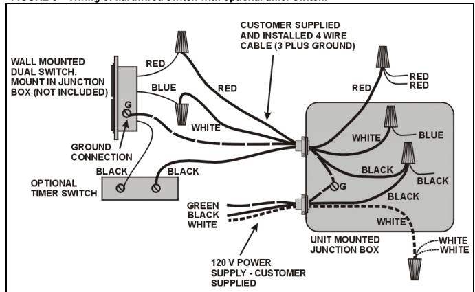
FIGURE 6 – Wiring of hardwired switch with optional timer switch.
