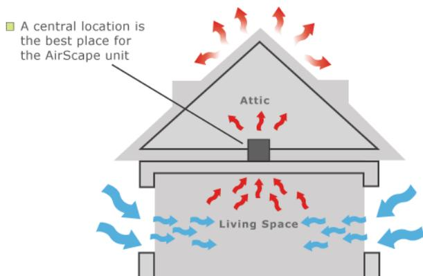
Installing the unit centrally ensures air is replaced evenly throughout your house
