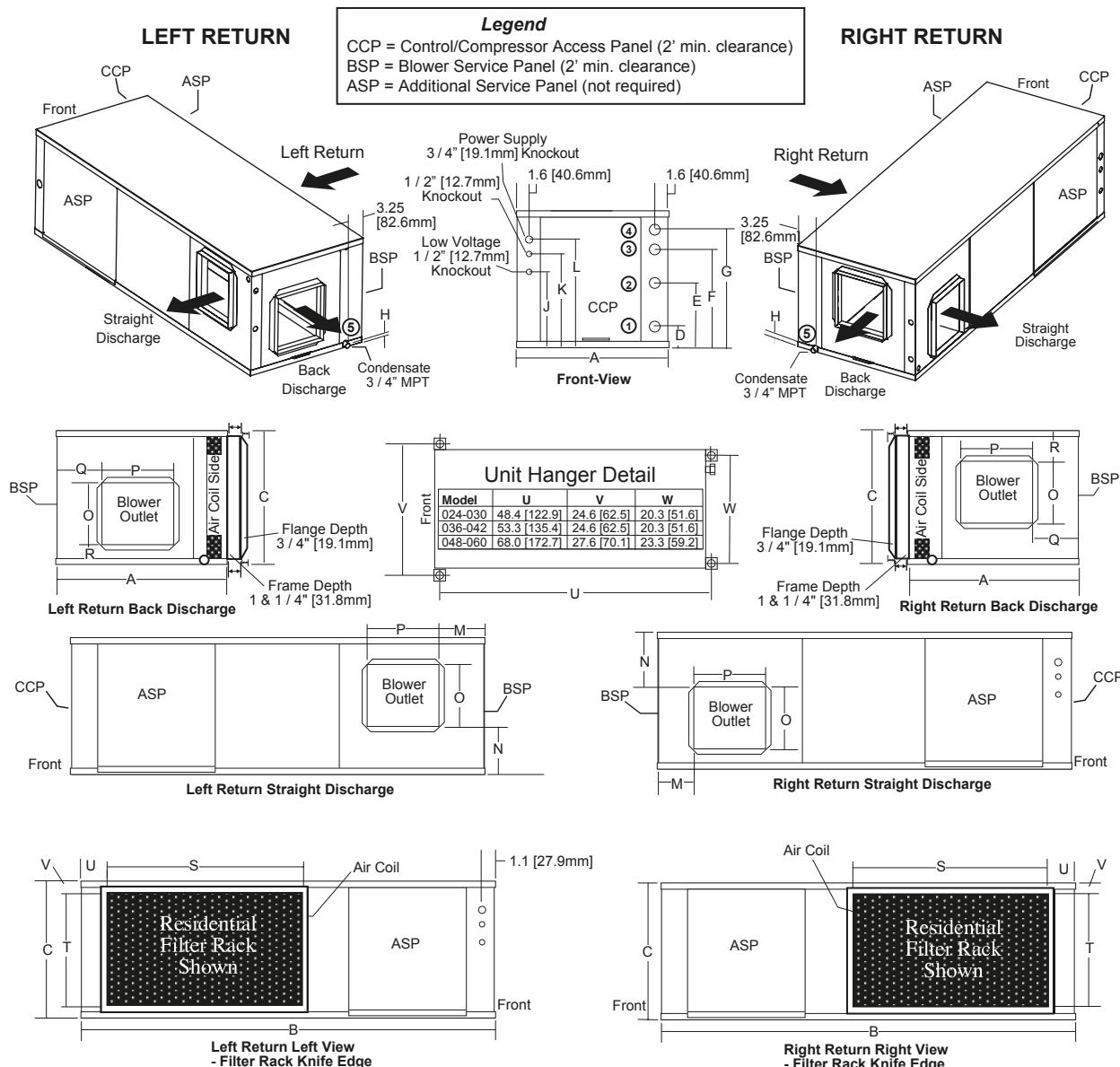
Note: Provide 2' minimum clear access to the Control/Compressor Access Panel and the Blower Service Panel.
