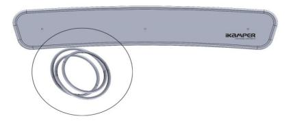
Take rubber strap [B] and wrap it around panel [A]. The harder rubber side should be facing the front of panel [A] with the iKamper logo, with the softer rubber side facing the back.
