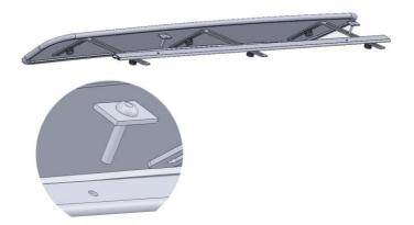
Insert the 2 bolts [H] in the holes on top of rail [D]. The wider sides (35mm) should be facing the front and back of the rail. Loosely screw on head nuts [G].
