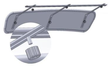
Place rail [D] over the 3 metal pieces [C], insert the 3 bolts [F], and screw on the 3 head nuts [G]. The thicker end of rail [D] should be facing panel [A].
