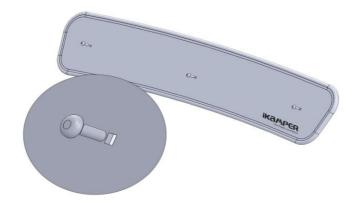
Insert 3 bolts [F] into the front of panel [A].
