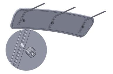
Take metal piece [C] and place the short side over bolt [F]. Then screw on head nut [G], and repeat for the other two bolts.
