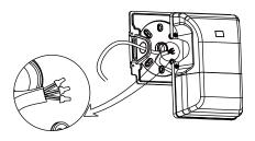
8. Turn on the power after make sure good wiring and insulation
