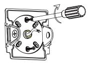
7. Fix the fixture by 4 screws
