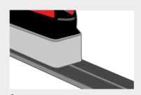
For extra durability: Iron the first layer of wax into the base. This process will increase contact between base and wax. Temperature setting of the iron is approx. 100°C.
