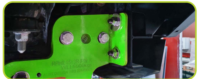
Figure 10 - RPHIL15v3 Fitted with Opposite Lock Rear
