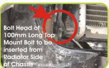
Ensure all supplied and specified components are used during the installation of tow points. Failure to do so will significantly reduce the Working Load Limit (WLL) specified for each individual point (5000kgs), which can result in serious injury or death.
