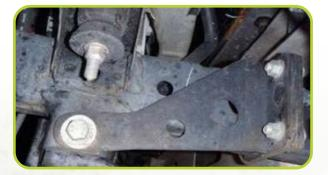
This is the mount from a Genuine Bull Bar. This mount strap uses the bolt hole (below the shock mount) that is required by the tow point. It also conceals the third hole required for correct tow point mounting. **NOTE:** Due to the **O5**-on Hilux chassis design, it is imperative that two points are used in conjunction with each other via a bridle strap. This is to avoid damage or unnecessary strain to the chassis, which can increase fatigue causing possible chassis failure.
