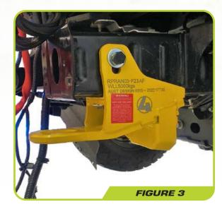
All bolts to be tightened to the appropriate torque value based on nominal size, pitch and grade, or OE manufacturer's specs.
