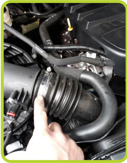
17. Loosen the hose clamp on the air filter lid and outlet and reposition to take strain out of the hose.
