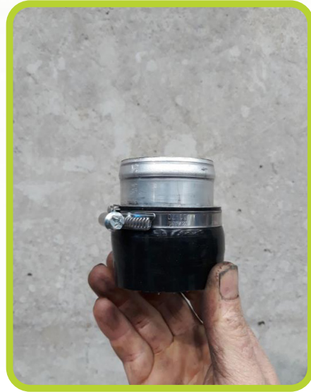
18. (3.2L Engine) Loosen the right hand intercooler hose on the bottom (near power steering pump). This extension will need to be fitted once lifted.
