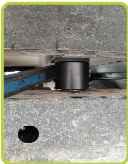
3. Loosen all tray mounts, remove left hand inner guard and check fuel filler/breather hoses and looms for enough length. Using a bar, lift one side at a time and fit the new spacers and bolts.
