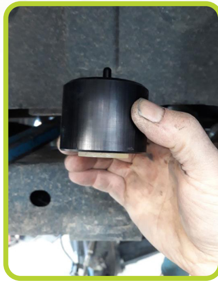
2. New 2" spacer with OE rubber packer ready to be installed.
