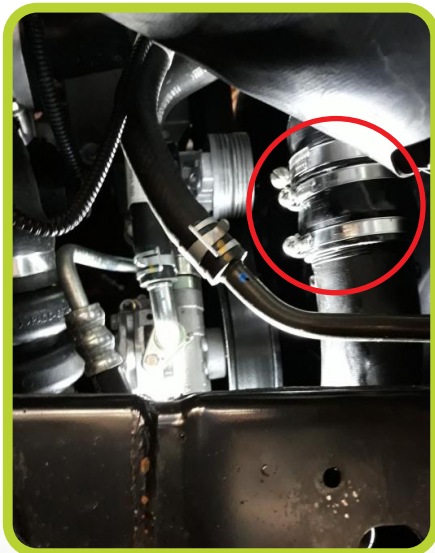
19. (3.2L Engine) Extension fitted to the right hand intercooler hose seen through the right front inner guard.
