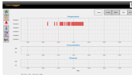
Conditions that put the Miri® into alarm state are recorded. It is possible for the software to send email alerts as well.
