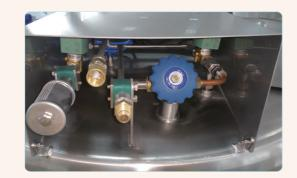
The unique design can reduce the amount of water vapor solidification on the outer surface of the neck, the container is reinforced at liquid nitrogen temperature to extend the physical service life of the container.
