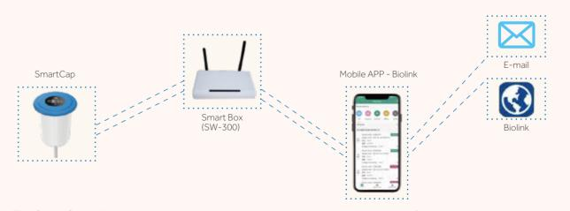
The SmartCap collects liquid level data and temperature data and transmits the information to cloud data store wirelessly, via 2.4G at a fixed interval every 10 minutes. Users can check real-time data and system alarm situation at any time through the Haier mobile APP-Biolink.
