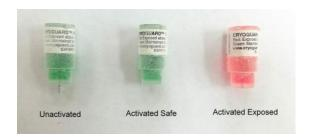
Each indicator is a chemical formulation sealed in a plastic vial that is approximately ½" in diameter and 1" tall. The indicator when green verifies, in real time, that monitored heat labile material has never suffered damaging thermal exposure.
