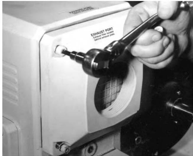
**Fig. 3 - Removing the Exhaust Housing**
