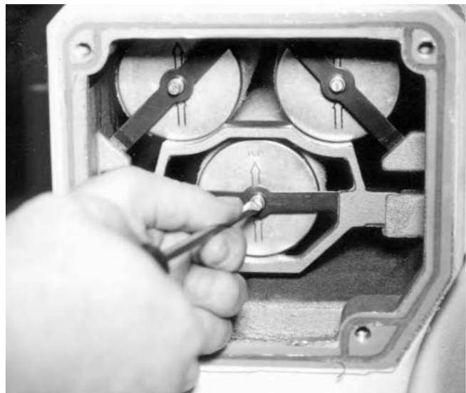
**Fig. 4 - Removing the Filter Spring**
