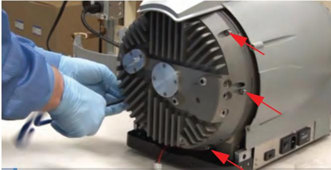
1. Use an 5 mm Allen key to remove the six screws on the outboard housing (the three screws on left not shown). Remove the lower screws first to support the housing.
