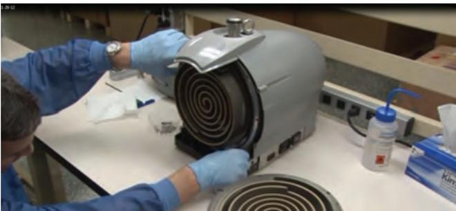
4. Lightly lubricate the O-ring with a trace of vacuum grease. Use the Krytox 224 grease supplied with the kit. Krytox LVP or Apezion L can be substituted. Do not use vacuum grease containing silicone.
