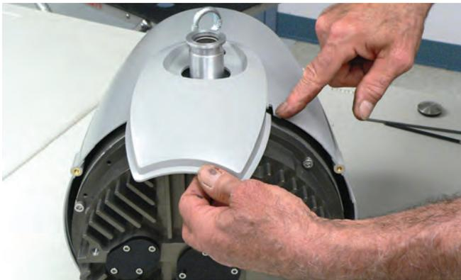
3. Reinstall the console by swinging it back and aligning it with the body slots as shown.
