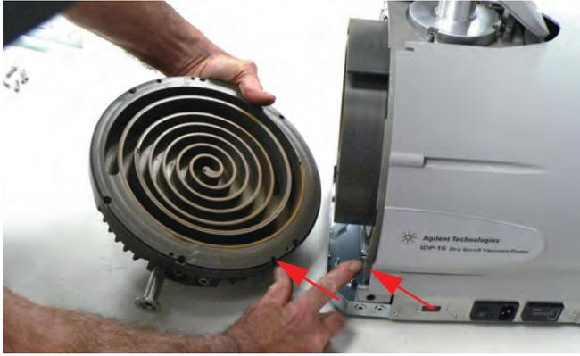
1. Align the outboard housing with the orbiting plate using the pin and pin alignment hole shown by the red arrows. Ensure that the tip seals and O-ring do not get pinched or misaligned.
