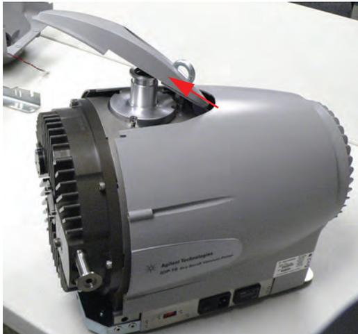
10. Lift the top console (red arrow) from the front and rotate to one side.
