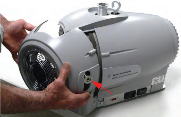
5. Rotate the cowl so that it clears the exhaust port (red arrow).
