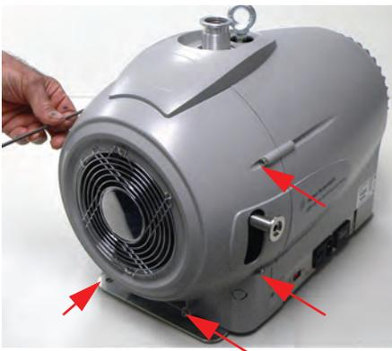
2. Remove the two screws holding the bottom bracket using a 4 mm Allen key.
