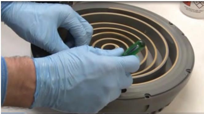
4. Using a pry tool, remove the old tip seals. There are a long and short tip seal on both the orbiting plate and the outboard housing.
