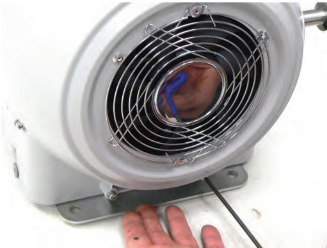
4. Place the bracket against the electrical tray and align the bracket slots with the tapped holes in the tray.
