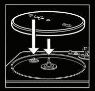
SET THE SLIPMAT ASIDE AND PLACE THE PLATTER ONTO THE TURNTABLE.
