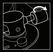
ONCE ALIGNED WITH THE CORRECT GROOVE, TURN THE TOP SCREW CLOCKWISE TO TIGHTEN THE COUNTERWEIGHT.
