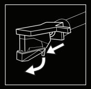
ORTOFON 2M SERIES: (VPT-2500) PUSH THE STYLUS COVER TAB DOWN / FORWARD AND GENTLY SLIDE THE COVER OFF.
