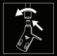
INSERT THE HEADSHELL INTO THE TONEARM AND TIGHTEN THE TONEARM COLLAR COUNTER-CLOCKWISE UNTIL THE HEADSHELL IS SECURE.
