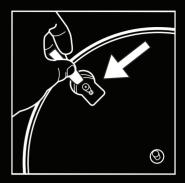
CAREFULLY REMOVE THE TAPED GUIDE STRING AND USE THE STRING TO STRETCH THE BELT OVER THE MOTOR SPINDLE.
