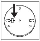
FIND THE GUIDE STRING TAPED TO THE PLATTER AND CAREFULLY REMOVE THE TAPE WHILE HOLDING THE STRING
