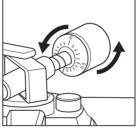
HOLDING <u>BOTH</u> THE NUMBER RING & COUNTER WEIGHT, ROTATE <u>COUNTERCLOCKWISE</u> 1 1/2 ROTATIONS UNTIL YOU END ON "1", THAN TIGHTEN SET SCREW
