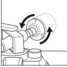
SET <u>ONLY</u> THE "NUMBER" RING, SO "0" IS IN THE TOP MOST POSITION: <u>DO NOT LET</u> <u>THE REAR WEIGHT TURN</u> (NUMBER RING AND COUNTER WEIGHT MOVE SEPARATELY FROM EACH OTHER)
