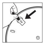
USE THE STRING TO PULL THE BELT OVER THE MOTOR PIN -ONCE BELT IS ON MOTOR PIN, DISCARD THE GUIDE STRING
