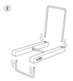
INSERT THE TALL BAR INTO THE TOP HOLES IN THE BACK OF THE STAND. INSERT THE SHORT BAR INTO BOTTOM HOLES IN THE FRONT OF THE STAND.
