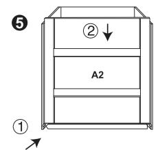
**STEP 5:** 1. Make sure C is pushed all the way forward into the slots of B2, A1, & B1.
