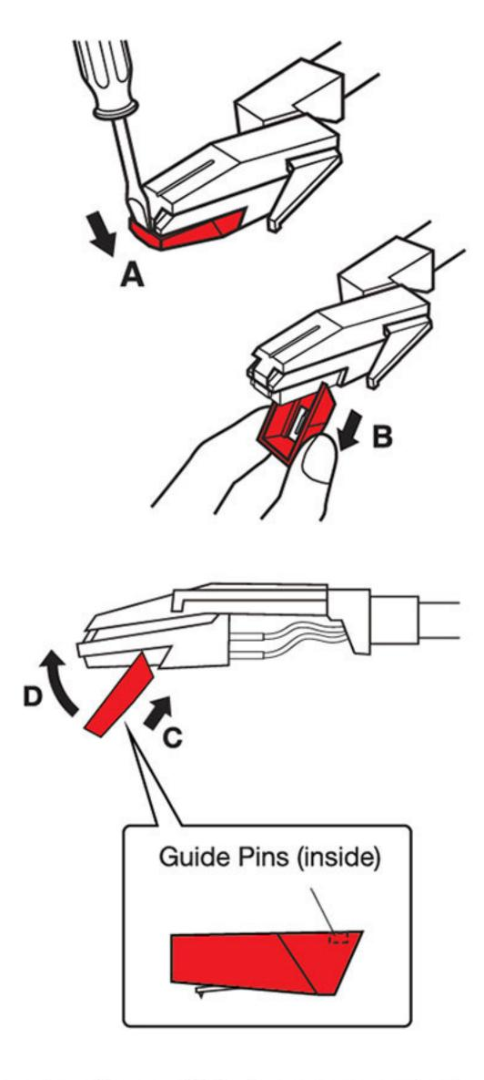
Please note: The stylus should last about 50 hours under normal use. It is recommended that the stylus be replaced as soon as you notice a change in sound quality. 78 RPM records may accelerate stylus wear and may have to be changed sooner.
