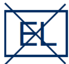
Lamp not suitable for emergency operation
