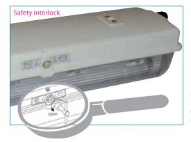
The light fitting is equipped with an interlock device mechanically connected with the internal Ex de safety switches, that automatically cut-off the power when the enclosure is opened.
