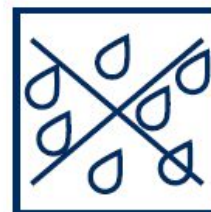
Lamp to be used in dry conditions or in a luminaire that provides protection
