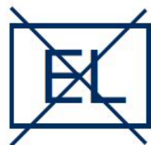
Lamp not suitable for emergency operation
