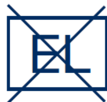
Lamp not suitable for emergency operation
