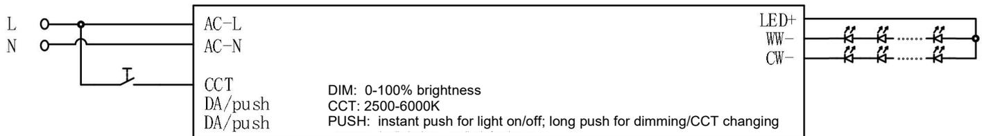
**⚠ Remark: Before using PUSH dimming function, please connect AC-L/AC-N to electricity FIRST, then connect the CCT terminal to electricity. Otherwise the CCT terminal will be burned.**
