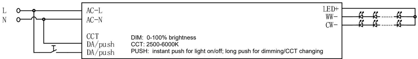
**⚠ Remark: Before using PUSH dimming function, please connect AC-L/AC-N to electricity FIRST, then connect the PUSH terminal to electricity. Otherwise the PUSH terminal will be burned.**
