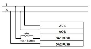
A Remark: Before using PUSH dimming function, please connect AC-L/AC-N to electricity FIRST, then connect the PUSH terminal to electricity. Otherwise the PUSH terminal will be burned.
