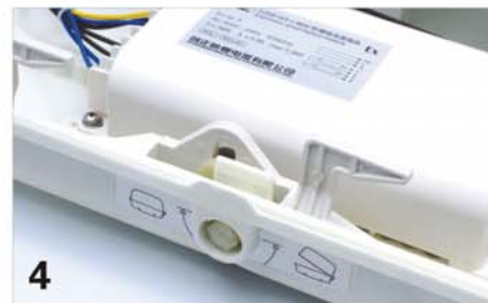
The enclosure and transparent shield are pressed tightly and drive the switching off and interlocking function of explosion-proof distance switch by unlocking device through interlock mechanism.
