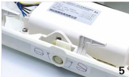
The enclosure and transparent shield are pressed tightly and drive the switching off and interlocking function of explosion-proof distance switch by unlocking device through interlocking mechanism
