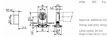
L1-4: Recommended dimension - The distance between the cut-outs and the tolerance should be governed by the dimensions of the respective lamps and luminaires.
