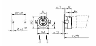
L1+27.0: Recommended dimension is based on use of one lampholder with and one lampholder without spring. The final distance should be governed by the dimensions of the respective lamps and luminaires.
