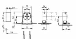
L1-1 / L1-6: Recommended dimension - The distance between the cut-outs and the tolerance should be governed by the dimensions of the respective lamps and luminaires.
