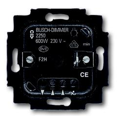
With rotary control, 2way On-Off switching and soft-catch. Leading Edge control. For incandescent lamps and 230 V tungsten halogen lamps. With adjustable minimum brightness. Without cover plate.
