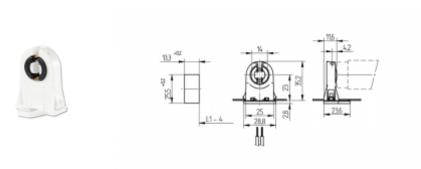
L1-4: Recommended dimension - The distance between the cut-outs and the tolerance should be governed by the dimensions of the respective lamps and luminaires.
